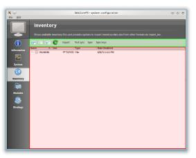
The inventory panel allows to import and synchronize inventory files. It shows a list of inventory XML files located in folder etc/inventory.
